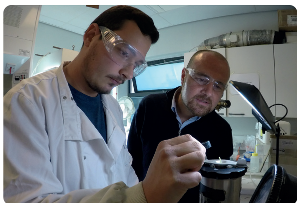
Image 1: Measuring plant water potential in a pressure chamber.
